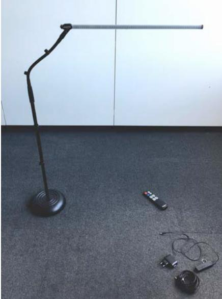
A photograph showing the gooseneck device mounted on the tripod stand. The gooseneck is bent at a 90-degree angle. On the floor in front of the stand, there is a small black remote control, a coiled black cable, and a small black device.             | <p>Step 5:</p> <p>Turn the gooseneck 90 degrees. In this position, insert the stimulation unit of the REMSTIM 4000 into the clamp so that the tube protrudes only a few mm on the side of the socket for the power connection.</p>                     |
