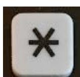
The star key is the second most important key and controls the focus functions 1 and 2. Both focus functions end automatically after 30 seconds, if you have not previously stopped them by pressing the red key, ie by starting a stimulation sequence, or actively be terminated.
