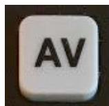
The AV key allows during a stimulation sequence to switch back and forth between the stimulation signal duplicated on the back and the reduced clock signal.
